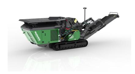
This versatile, mobile crusher is able to nimbly move around in small spaces, and continue moving while crushing. The I3C's small footprint is uniquely suited to the demolition and asphalt recycling, aggregates and smaller scale construction projects. Less than 2.5m wide, the crushers can be transported easily from site to site.
