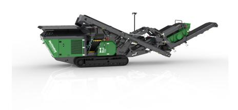
This versatile, mobile crusher is able to nimbly move around in small spaces, and continue moving while crushing. The I3C's small footprint is uniquely suited to the demolition and asphalt recycling, aggregates and smaller scale construction projects. At just over 2.5m wide, the crushers can be transported easily from site to site.
