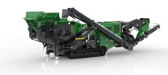
The large 1060mm (42") x 700mm (28") jaw chamber accommodates large feed sizes, contributing to higher production in material processing. The material path can be enhanced with an optional double deck 1064mm x 2215mm (41.9" x 7' 3") double deck grizzly prescreen under the hopper that, along with the variable speed pan feeder, allows for better sizing of material with a variety of mesh options.
